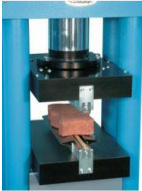
Interlocking Paver PSI Compression test
