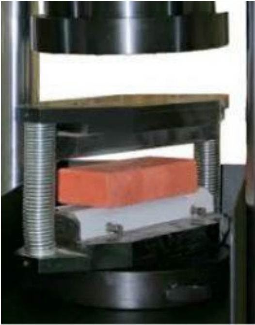
Tensile Interlocking Paver Strength Test
